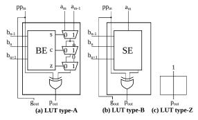
Fig. 5. Configuration of LUTs used in proposed methodology
