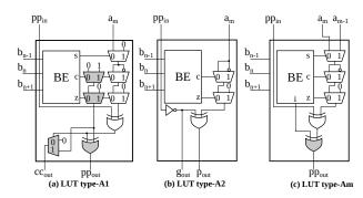
Fig. 7. Modified configuration of LUTs
