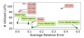
Fig. 13. Design space showing the area-accuracy trade-off of different designs for an  $8\times 8$  multiplier (Pareto points are in green).
