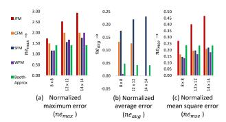
Fig. 12. Comparison with truncated and rounded multipliers: JFM [35], CFM [36], SFM [37], WFM [34]
