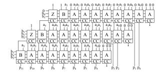
Fig. 6. A 6×6 accurate multiplier implementation (Booth-Mult)
