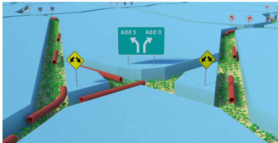
Fig. 1: Split junction overview. Illustration of protein filaments (red) propelled by molecular motors (green) arriving at a junction where they perform a calculation operation (adding 5 or adding 0).
